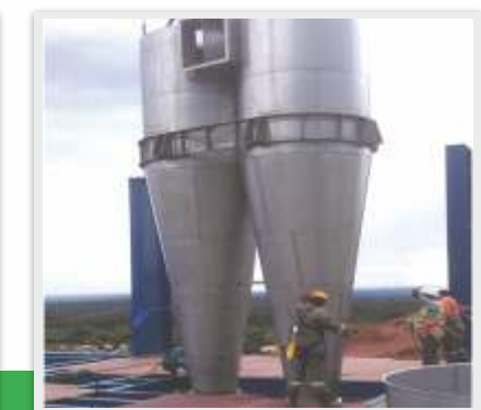
Twin Cyclones For ASFD, Mutanda Mining SPRL, D R Congo
