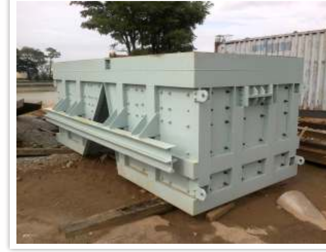
Fabricated bulk head chute for Rocker breaker @ Konkola Deep mining project, Chililabombwe
